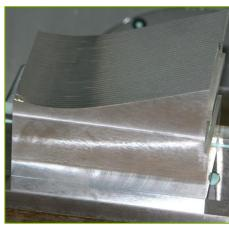
Surface Patch based CNC cutter path; special CNC smoothing function used
