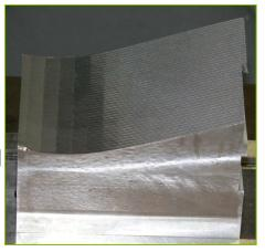
Mesh based CNC cutter path; special CNC smoothing function used
