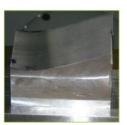
Auto-Surface based CNC cutter path; special CNC smoothing function used
