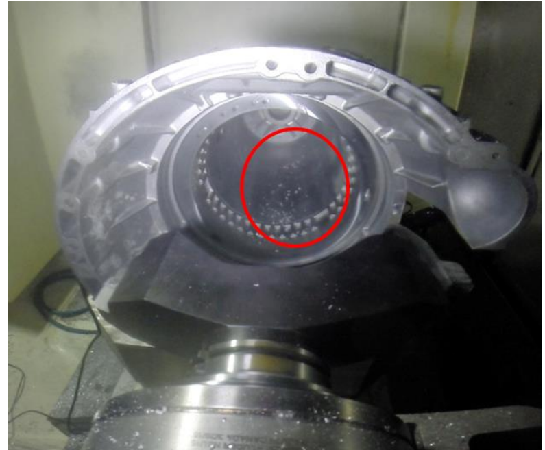
Chips in part after early test on RWD transmission main bore
